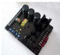
Caterpillar Generator AVR VR6 K125-122 K125-10B
